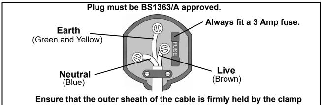
We strongly recommend that this machine is connected to the mains supply via a Residual Current Device (RCD)
